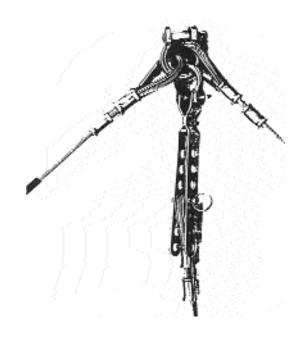
Attach your existing 10-hole adjuster to the upper pigtail as shown.
