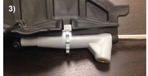
3) Place part in position on spine. Slide shaft in from forward end toward aft through part. This pushes foam out.
