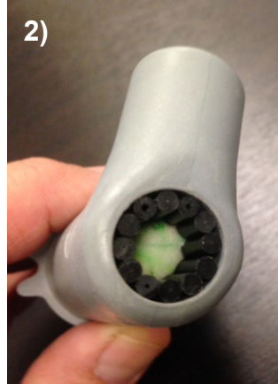
2) Remove adhesive strip. Note foam plug inside.
