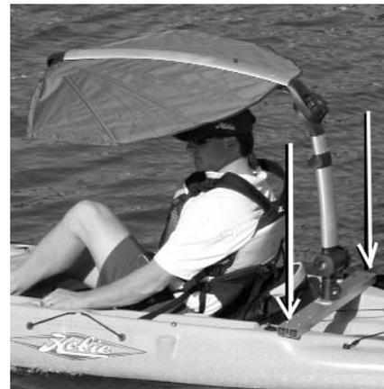
You will notice that the mount is adjustable. There are two screws on the bottom of the mount that when loosened, allow the outer sections of the mount to move. Adjust the mount so that the ends of the mount sit firmly on the kayak and the mounting holes are fairly centered over the rails. Once it is adjusted properly, tighten the screws on the bottom to hold the sliding sides in place.
