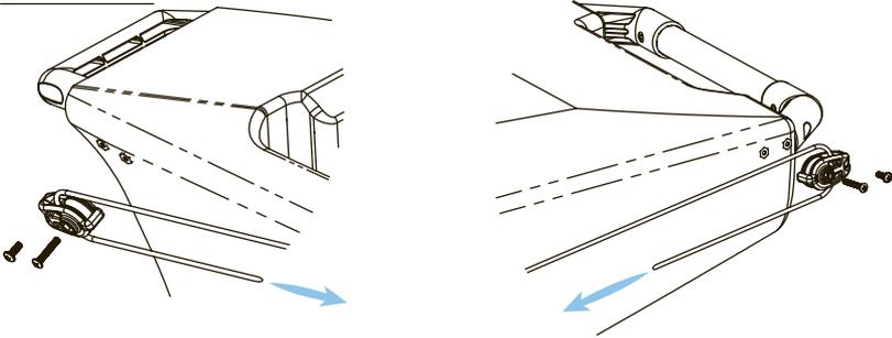
Install cheek blocks to boat using the 1" and 1/2" screws. Make sure the blocks are facing inwards. Feed the Trolley Line through the top of the blocks and exit the bottom. Tie each end of the line to the rings on the shock cord. The shockcord assembly should travel on the bottom trajectory. Make sure there is tension in
