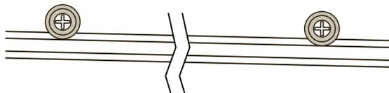
For Pro Anglers without inserts, drill two 3/8" holes per the diagram below.
