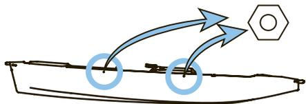
If you have two molded inserts on the side of your boat, mount the eyelet posts to the inserts. You will need to take apart the well nut assembly and use the eye post provided. Use the 10-32 X 3/4" Flathead screw. Place a drop of Loctite on the threads.
