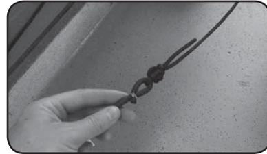
8. Just behind (approx 8"-12") where you tied the line to the Bungee® loop, feed the line through the plastic hook as shown in the diagram. The line may be a little tight going through the slot. If it is, use a small flat-head screwdriver to help push the line through.
