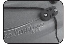
7. Take the end of the line that passed through the rear block and tie it through one of the looped ends of the Bungee® cord.
