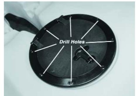
5. Press the attachment screws through the top of the hatch and into the hull. Grab the backing ring that you put into the hull and align the holes in the ring to the screws. You will want to start to thread each screw into the backing ring before tightening it down all the way. Make sure that the screw is entering the side of the ring that is flat....not the side with the little cylinders of plastic.
