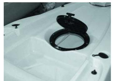
4. Once you have the hatch in the position you want, use the outer holes as a drill guide to drill 3/16" holes. As mentioned above, you may not need to drill any holes for the 6" hatch if it is located the way you want it.
