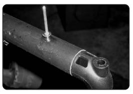
3. With the tiller crossbar, you only install a rivet in one of the holes. On the hole that is 1-3/16" from the end of the tube, turn the tiller end cap so that it is facing down and align the small hole in the plastic part with the hole in the aluminum bar. Thread the small sheet metal screw into the hole and tighten down. This will allow only one side to spin while the other is stationary.
