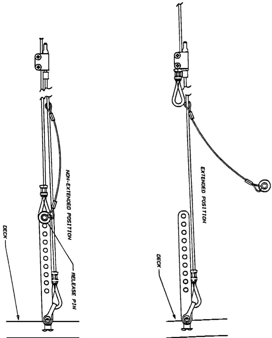
\* These drawing depict the shroud extender attached to the shroud anchor pin with a shackle. The written instructions are to install the shroud extender to the shroud adjuster with the clevis pin. Either method is acceptable.
