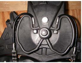
6A. Insert idler cable into rear slot as shown. Note -- this slot is divided -- use outboard portion of slot (left).
