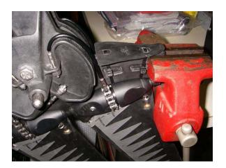
5 B. Mount the rear sprocket cable. Note, the cable is first inserted from the side, with the help of needle nose pliers if necessary, then re-routed over the top lip of the drum. Hand thread Nyloc nuts enough to keep the cable from slipping
