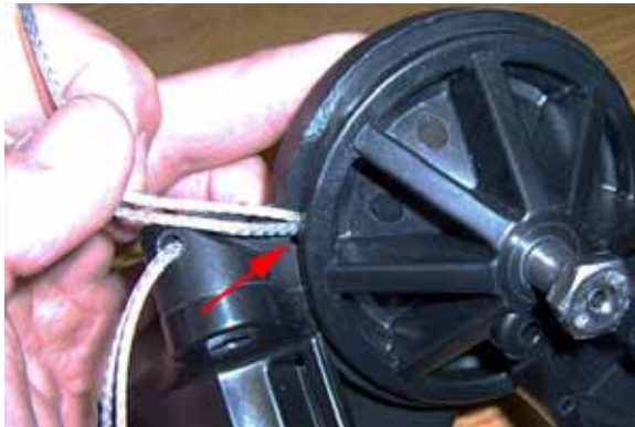
3) Hold the lines in the recess
