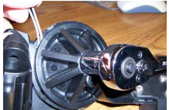
4) Tighten (9/16" wrench) until...
