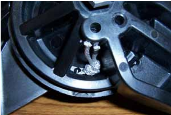
13) Slack in the system can be pulled out / adjusted here. Tension, knot and trim the lines. Pull the line slack forward to seat the knot.
