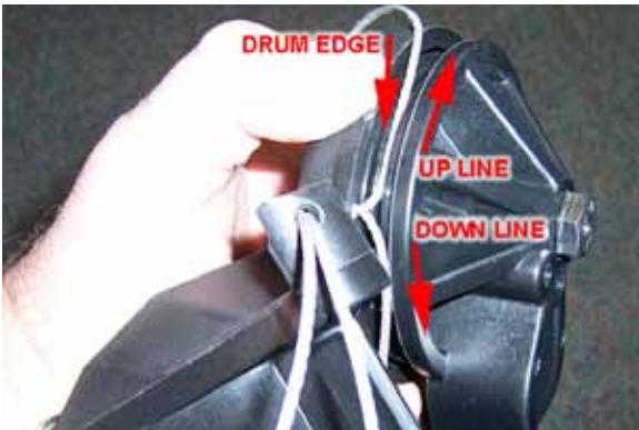
5) ...edge of drum is flush with housing
