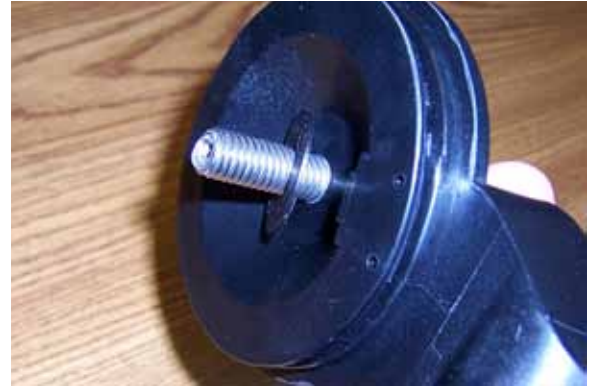
2) Re-attach the drum side (note washer)
