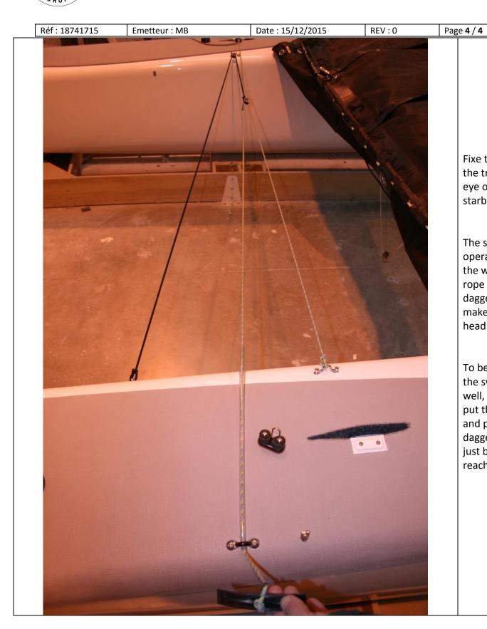
Fixe the elastic on the trampolin padeye on the starboard hull.
