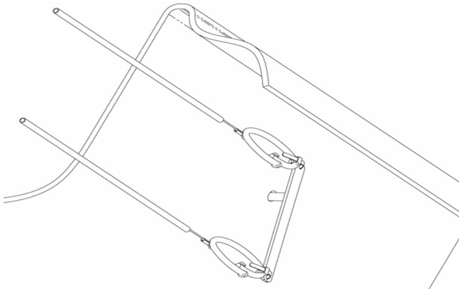
This crank doesn't have rivets, use a zip ties to attach the bungee to the cranks and bungee to the up/down control lines. If your up/down control crank does have rivets, use the small links and press the small loops over the rivet heads. Then use the zip ties to attach the bungee to the links and bungee to the up/down control lines.
