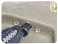
7. Thread the screws you just removed back into the holes so that they seal the hole. Make sure to lightly tighten the screws back into the holes so they don't strip out the plastic.
