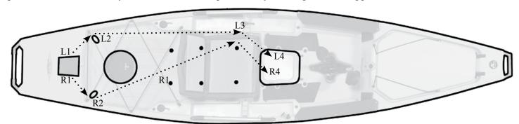
5. Bring the steering crank to the center hatch and loop the ends of the line over the rivet that is assembled to the crank. Note diagram to the right showing which line attaches to what side of the crank. Note the orientation of the "L" tab on the crank in the pictures.
