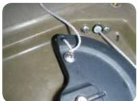
5. Follow the same procedure for the left steering line. The only difference is that it will wrap around the front of the drum and will come up through the hole on the right side of the drum.
