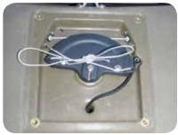
7. Put the cover back over the steering drum and place the Hobie sticker over the screw on the handle. You may need to tighten the lines after some use
