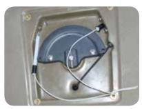
3. Press the small tube assemblies into the holes. It will be a snug fit, so you may need a small hammer to tap the tubes completely in.
