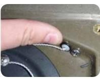
4. You will now feed the lines through the kayak up to the middle hatch. Follow the diagram to trace where the right (R) and left (L) lines need to pass. Be sure to note how the right lines pass through the cart and seat scuppers. This is the best way to route the lines to prevent any rubbing on the scuppers.
