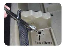
4. Using the provided screws and nuts, reach inside the boat and bring the crank support block up to the inside surface of the kayak. Install the screws through the bottom plate on the riser tube assembly, through the hull and crank support block. Place a nut on the end of the screw and tighten. Follow this procedure on all four hole locations to securely bolt the plate to the kayak. Clean up any excess silicone that squeezes out.
