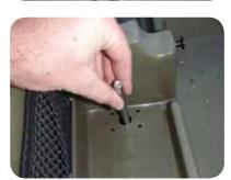
3. Slide the steering tube riser over the steering crank shaft and allow the plate on the riser assembly to sit flush on the hull. Place a small amount of silicone on the hull around all of the holes to provide a watertight seal.
