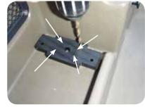
2. Using a pen or marker, trace a circle onto the kayak using the larger center hole as a guide.
