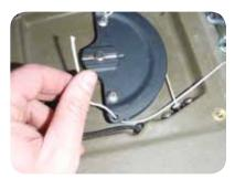
6. With both lines tightened under the screw heads, try the steering and make sure it is adjusted to your liking. You can adjust the lines to remove excess slack as desired. Tie up the extra line to bunch up the slack.
