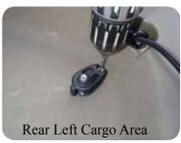
2. Take the pulleys off the boat and re-drill the holes with a 7/32" drill bit to enlarge the holes.
