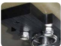
5. Use a 7/32" drill bit to drill two more holes for the upper support on the tube riser. The strap that goes around the tube will be your guide for the holes. Be sure to drill the holes all the way though both sides of the scalloped rod holder on the kayak. Be sure to drill the holes as straight as possible.
