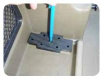
3. Find the center of the hole you just traced and drill a 5/8" hole.
