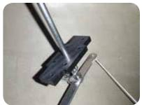
2. Feed the long shaft of the steering crank through the 5/8" hole you drilled into the boat. Be careful to bring the steering crank straight back and don't twist the lines. Inspect the lines and make sure they are following the path of the diagram on the previous page.
