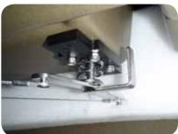
8. Place the handle on the steering crank shaft so that the pointier end of the handle faces forward and the pressed in-pin indexes to the pin profile on the bottom of the handle.
