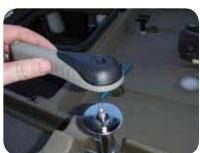
9. Once the handle is on the steering shaft, install the screw on the top of the handle to secure it in place.
