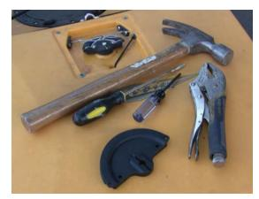
**Tools and Parts required.** The replacement drum, Phillips head screw driver, Blade screw driver, Vise grips, Hammer.
