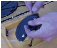
5) Thread the control lines into the new drum. Note that the lines cross when installing the lines on the drum. Left line routes to the right side of the drum. Right line to the left side. Press drum in place.
