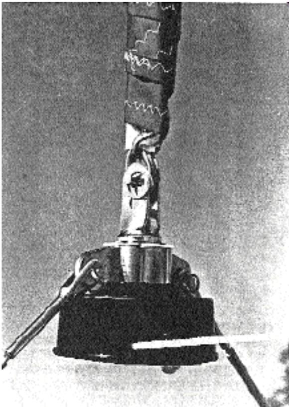
The jib luff wire is the forstay when using the roller-furling jib. Step your mast then attach the jib tack to the furler drum as shown. Pass one end of the furler line from the inside to the outside of the small hole in the furler (Bottom on Hobie / top of Harken). Tie a small knot then, wind the furler line into the drum by spinning the furler in a clockwise direction when looking from the top down. When furler is wound, the jib should be unfurled.
