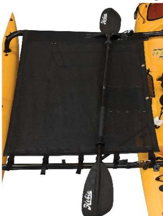
Another feature are the forward bungee straps for securing the trampolines while not in use. To use them unbuckle the rear of the trampoline, roll the material up toward the forward AKA and wrap the bungee around an onto the hook.
