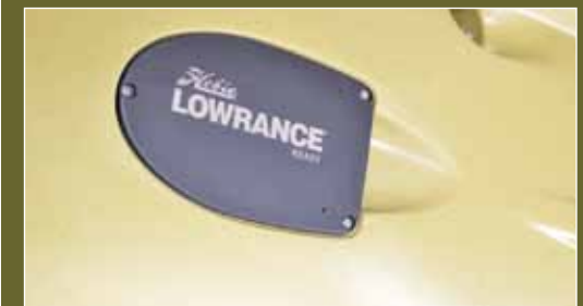
"Lowrance Ready" built-in transducer mount with pre-installed through-hull cable plugs
