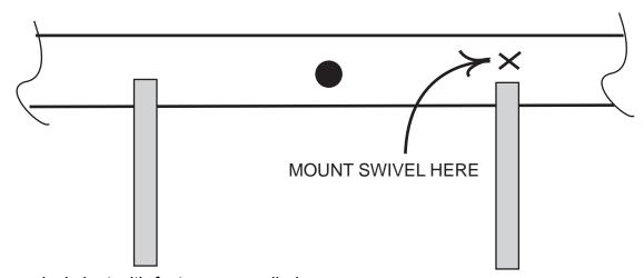
2) Fasten swivel cleat with fasteners supplied.
