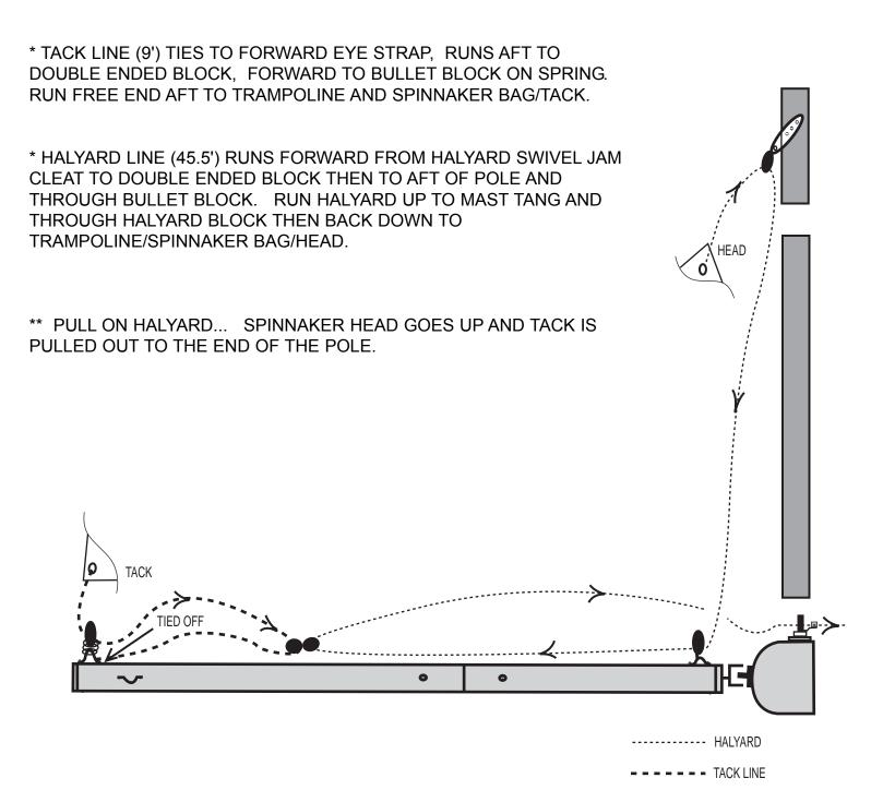
NOTE: BE SURE DOUBLE ENDED BLOCK CAN RUN FREELY, FORE AND AFT ALONG POLE. RUN TO STARBOARD OF BUNGEE SUPPORT. SPINNAKER SHEETS
